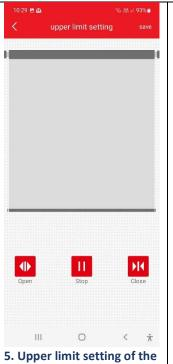
blind Hold Open or Close until the blinds is fully open, press Stop and Save.
