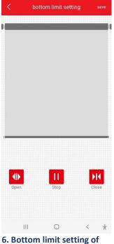
the blind Hold Open or Close until the blinds is closed completely, press Stop and Save.
